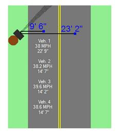
As vehicles pass the detection zone, the LiveView screen should show the speed and length of the vehicle.
