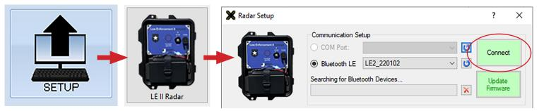
Select **Setup** from the Quick Start menu, then the LE II Radar. Make sure you have the "Bluetooth LE" radio button selected and click the **Connect** button to have the STARnext software connect to the Law Enforcement II Radar.
